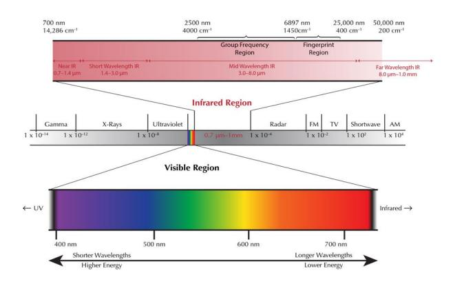
The IR spectroscopy concept can generally be analysed in three ways: by measuring reflection, emission, and absorption. The major use of infrared spectroscopy is to determine the functional groups of molecules, relevant to both organic and inorganic chemistry
